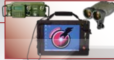
StrikeLink ® running on DRS's Military Ruggedized Tablet (MRT) which is outfitted with embedded SAASM GPS and tactical modem alongside tactical radio and Vectronix Vector 21B laser rangefinder.
